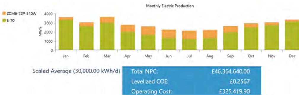
Figure 63: Monthly electric production by energy source, NPC, LCOE and operating costs for the off-grid wind, PV and battery one hectare system.
